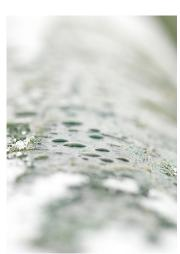
Timber treated with Copper Oil is green and fades over time.
